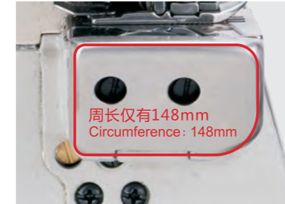
超小头148mm，缝制范围广 148mm small cylinder bed, wide range of application
