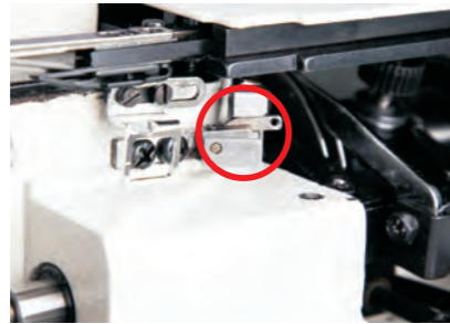
断线停车、底线不缠绕 Auto stop in case thread breakage, avoid of bottom thread enwinding
