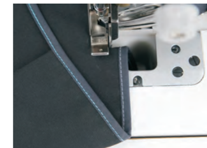
切包一体 ( BRC-5558G-T ) One machine with fabric edge cutter and tape binder functions
