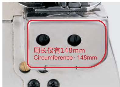
148mm small cylinder bed, wide range of application
