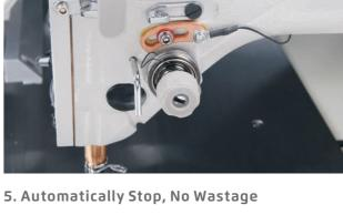
With the thread breaking sensor, machine will stop immediately in case thread breaking during sewing, do not damage fabric.
