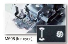
•The position of snaps can be changed in three stages from the center in a downward direction (maximum distance from the center : 10 mm).
