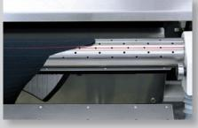
Laser beam for exact placing and positioning of the material
