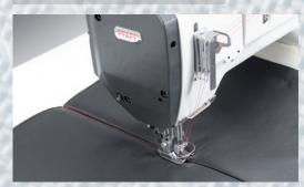
Double-needle top-stitching work on seat plates
