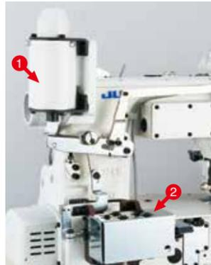
1 Presser lifter drive mechanism magnet
