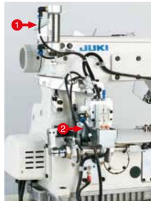
1 Presser lifter drive mechanism air cylinder
