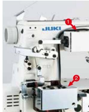
1 Presser lifter drive mechanism magnet
