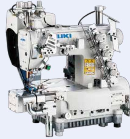
Semi-dry head, Cylinder-bed, Bottom Coverstitch Machine with digital type top feed / For hemming <with left hand fabric trimmer>
