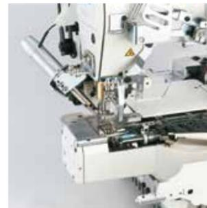
Electromagnetic needle thread / looper thread trimming device
