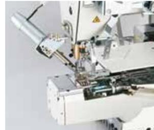
Electromagnetic needle thread / looper thread trimming device
