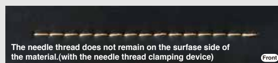
LU-1520NCS-7 (Remaining-thread length : Less than 5mm)
