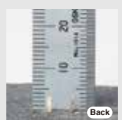
LU-1520NCS-7 (Remaining-thread length : Less than 5mm)
