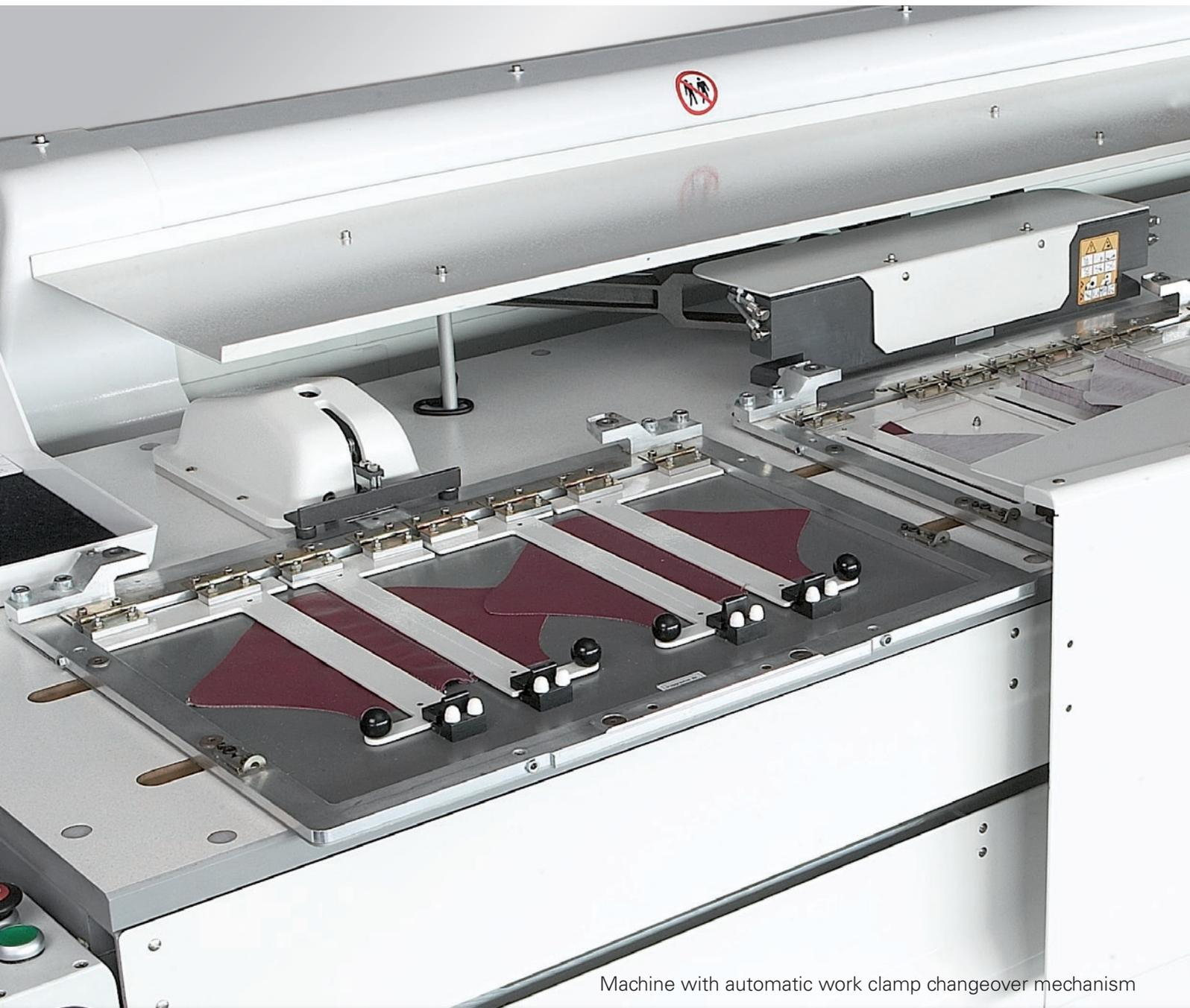
Machine with automatic work clamp changeover mechanism
