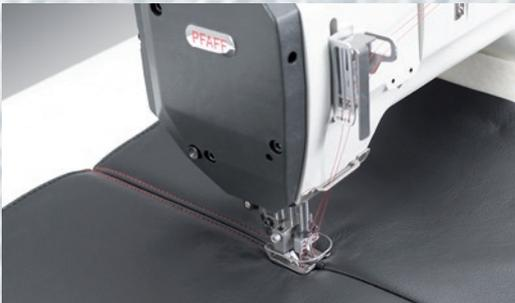
Double-needle top-stitching work on seat plates
